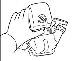
3. Push the primer pump several times until overflow fuel flows out in the clear tube. (OP3)
