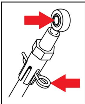
2. Unthread the heim joint (1) from the coupler (2), and then unthread the coupler (2) from the control rod (3). Discard the "unribbed" coupler.
