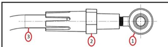
3. Thread the new ribbed coupler (2) onto the control rod (3) by hand until it stops (approximately 16 turns). Then thread the heim joint (1) into threaded coupler (2) by hand until it stops (approximately 19 turns).
