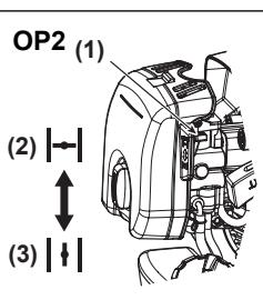
3. Move the choke lever to the closed position. (OP2)
