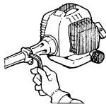
1. Each time before starting the engine, inspect the entire unit to see if every part is in good order and is securely tightened in place. If any damage is found in the fuel line, the exhaust system, or the ignition wiring, do not use the product until it has been repaired.
