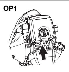
2. Push the primer pump several times until overflown fuel flows out in the clear tube. (OP1)
