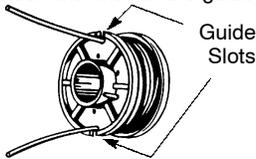
9. Insert the ends of the lines through exit holes in the sides of the trimmer head.
