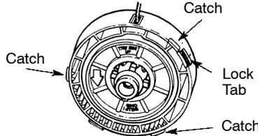
14. Make sure the lock ring is securely fastened by pulling on it and twisting in both directions.
