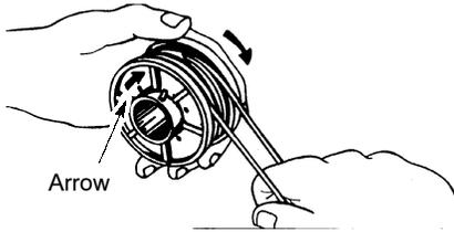
7. With your finger between the lines, wrap the lines evenly and firmly around the spool in the direction of the arrow on the spool.
