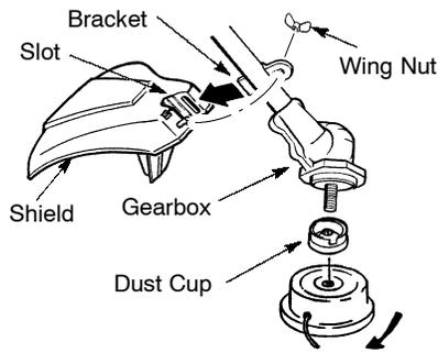
**NOTE:** Make sure all parts are properly installed as shown in the illustration before installing the trimmer head.
