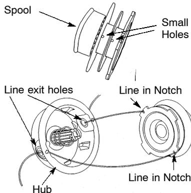
5. Wind the line evenly and tightly onto the spool. Wind in the direction of the arrows found on the spool.
