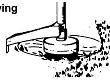
SWEEPING - The fanning action of the rotating line can be used for a quick and easy clean up. Keep the line parallel to and above the surfaces being swept and move the tool from side to side.
