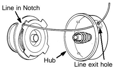
5. Wind the line evenly and tightly onto the spool. Wind in the direction of the arrow found on the spool.
