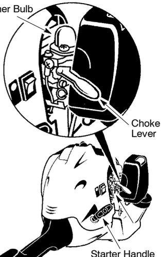
5. Pull starter rope handle sharply until engine sounds as if it is trying to start, but do not pull rope more than 6 times.
