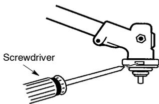
3. While holding the screwdriver in position, remove trimmer head by turning clockwise.
