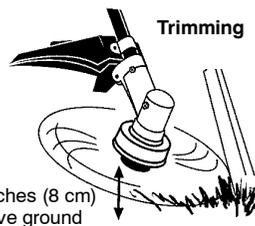
**SCALPING** - The scalping technique removes unwanted vegetation. Hold the bottom of the trimmer head about 3 inches (8 cm) above the ground and at an angle. Allow the tip of the line to strike the ground around trees, posts, monuments, etc. This technique increases line wear.
