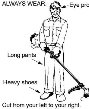
**WARNING:** Always wear eye protection. Never lean over the trimmer head. Rocks or debris can ricochet or be thrown into eyes and face and cause blindness or other serious injury.
