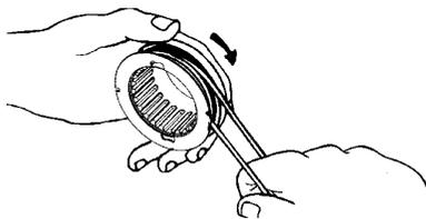
7. With your finger between the lines, wrap the lines evenly and firmly around the spool in a clockwise direction.
