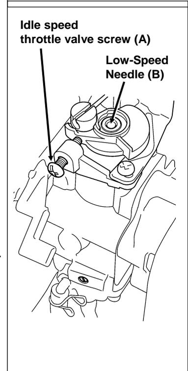
**NOTE: The initial carburetor settings for throttle valve idle speed adjust screw and Low speed mixture needle are intended to start and run the engine before final carburetor adjustments are made. Actual turns required for starting engine may vary slightly.**
