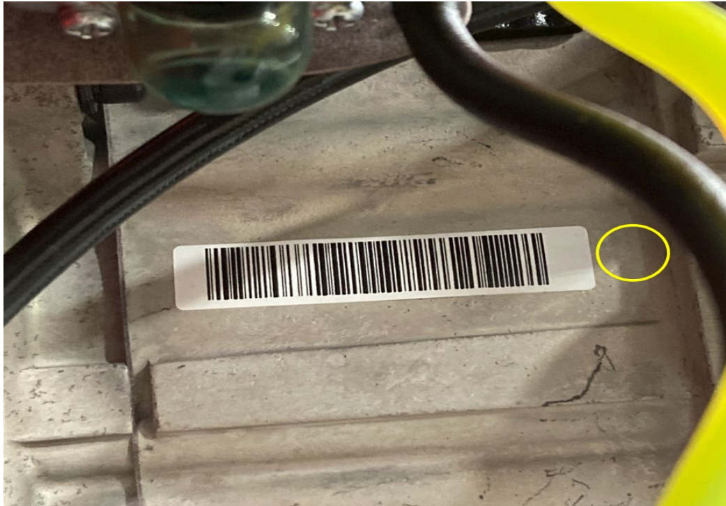
Figure 4: Position for punch mark on crankcase.
