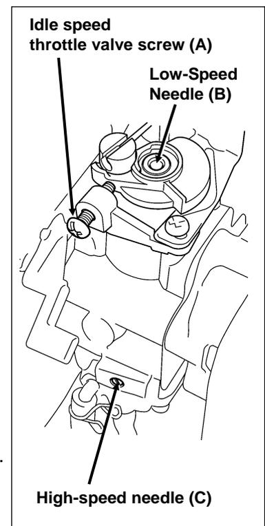
Start and run the unit to warm up the engine. Engine must be at operating temperature before completing Low speed mixture and High speed mixture needle adjustments. Warm up engine for minimum of 3.5 minutes by alternating between Wide Open Throttle (WOT) for 1 minute, then idle for 10 seconds.
